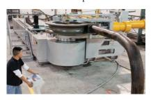
With state-of-the-art CNC large- and small-capacity bending equipment, as well as all complementary pipe end finishing equipment, the CPS team expertly manufactures *prefabricated piping assemblies*.
