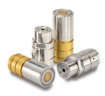
DSB Series balanced couplings have no hydraulic separation force while under pressure. The PEEK seals are durable for connecting at full system pressure. \*\*\*
