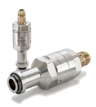
DSS Series swivels provide an unobstructed flow path. The force balanced design and low friction PTFE slipper seals minimize rotation torque. These features minimize pressure loss, can increase hose life and reduce fitting loosening.
