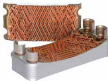
Fig. 4. A cut-away showing the cooling elements of the Parker OAW brazed-plate heat exchanger.
