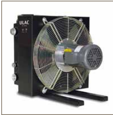
Fig. 2. Air oil coolers use surrounding air to remove excess heat. Specially designed fins promote turbulent air flow to improve heat transfer capability.
