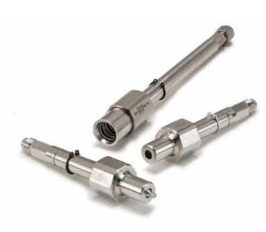
DSH Series couplings are used on subsea and topside RBQ/J - Plates. Typically found in hydraulic pilot applications they replace legacy couplings, pipe nipples, and fittings eliminating potential leak paths and reducing assembly time. The superior valve design of the DSH Series accommodates plate flex up to 0.100 in/2.54mm.
