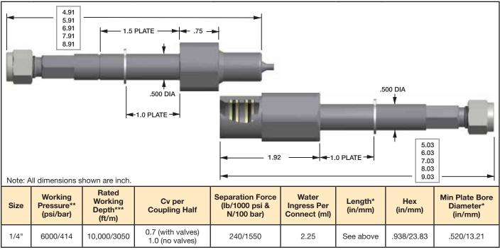
Data given is representative of the coupling series. Individual couplings may vary based on specific configuration of fittings/optional features. \*Minimum bore diameter and length are reference. May change for a specific plate configuration.
