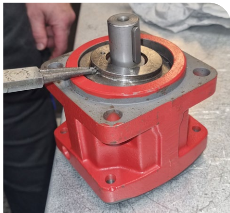
9. Remove the seal carrier (item 231)
