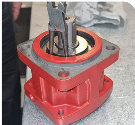
8. Disassemble the retaining ring (item 237)
