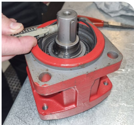
10. Remove the O-ring (item 225) Always change seal kit when removing seals.
