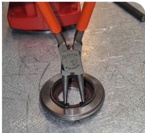
28. Assemble the retaining ring (item 238)
