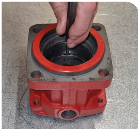
18. Tap the large bearing ring with a mandrel and hammer
