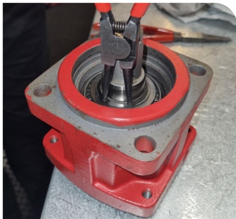
13. Disassemble the retaining ring (item 478)
