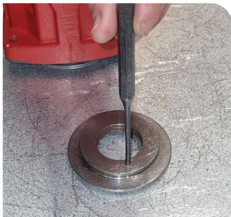
12. Tap the shaft seal out with hammer and mandrel.
