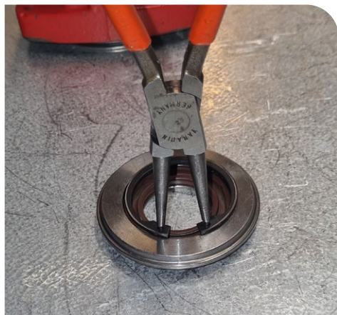
11. Disassemble the retaining ring (item 238)
