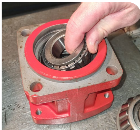
16. Remove the small tapered roller bearing (item 470)
