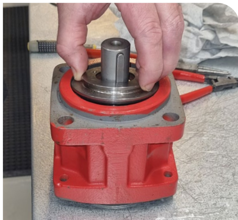
29. Install the seal carrier (item 231)
