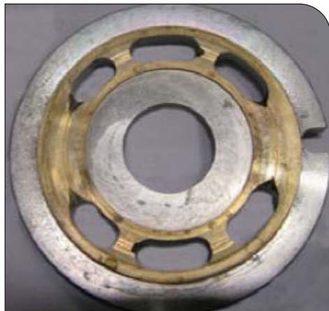
Valve plate with scratched surface.
